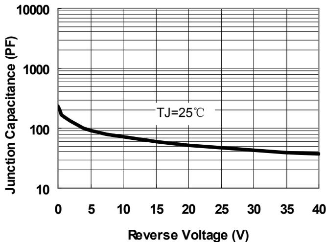
Fig.1-Typical Junction Capacitance
